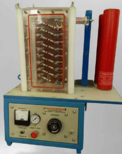
Forced Current Generator Z/34/139
