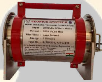
nsec Generator Z/51/146
