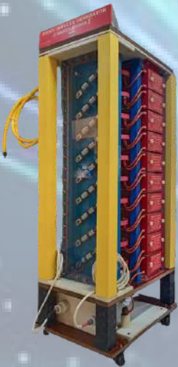
500kV Impulse Generator Z/36/66
